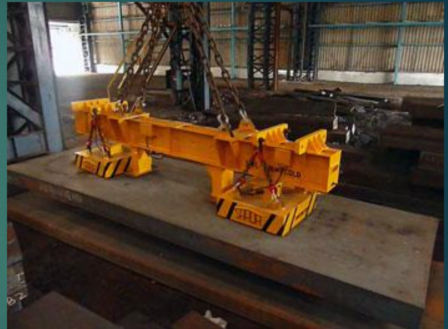
Figure 13: Industrial application of electro permanent magnets [9]
