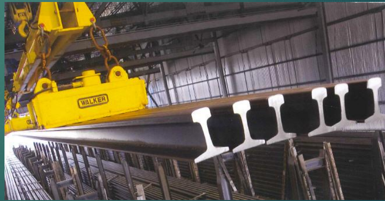
Figure 35: Industrial crane using electro permanent magnets [19]
