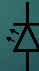
Figure 20: symbol for LED
