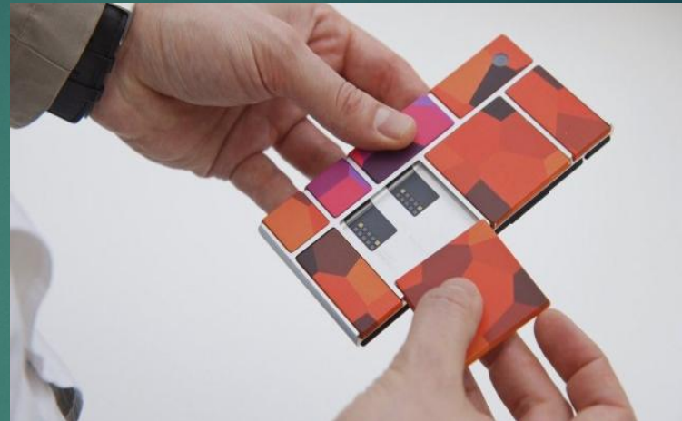
Figure 37: Consumer phone using electro permanent magnet attachments. [23]
